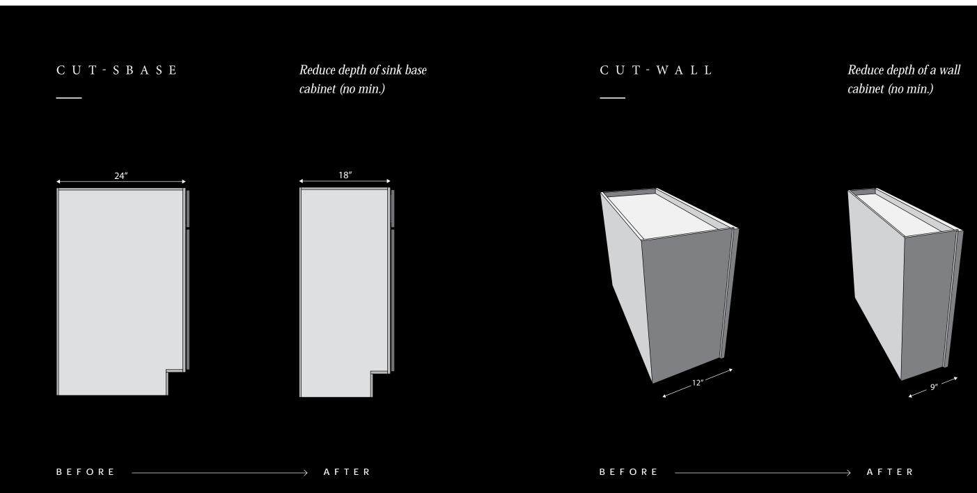
As with cabinet base and drawer base, the standard sink base comes 24" deep. Fabuwood will modify the depth to customer specifications. Modifications are done in 3" increments but can also be done in custom sizes such as 16" and 17" deep.
