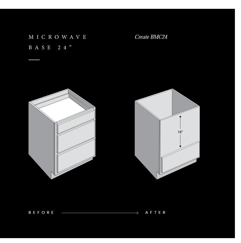
A 24" drawer base is modified to create a 24" microwave base. First, the top two drawers are removed. A support shelf is built on top of the bottom drawer, and a full flat panel is applied to
